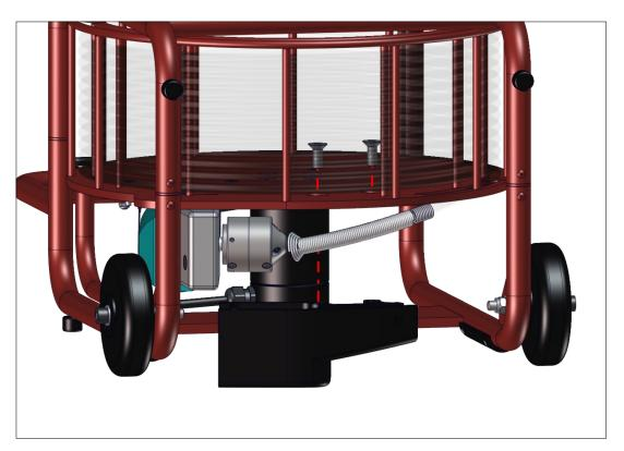
Step 9. During the final step, drill a 6.5mm/1/4" hole for the Strain Relief Lock so you can get the M6x25mm Bolt through the Miller's Reel Plate.
