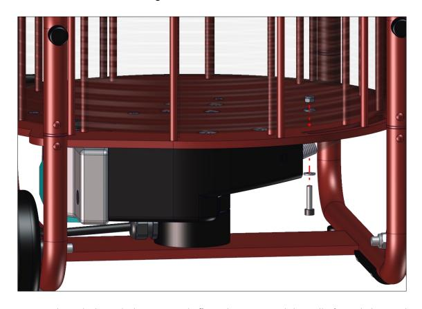
Step 10. Put the Bolt through the Strain Relief`s Locking Ring and the Miller's Reel Plate and tighten it using a Hex Key 5mm and a smooth jaw adjustable wrench 10mm.
