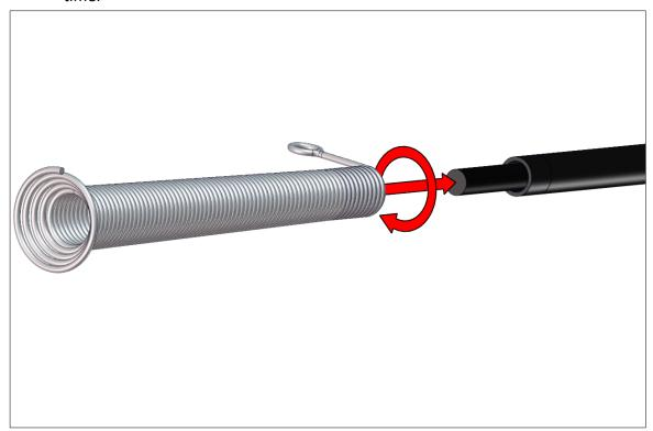
Step 4. The Outer Casing have to come through the Strain Relief Spring. This is really important part of STEP 5.
