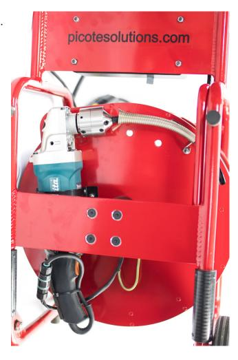
Step 8. Add the Hand Guard and tighten it with two M10x25mm bolts. Use a Hex Key 6mm.
