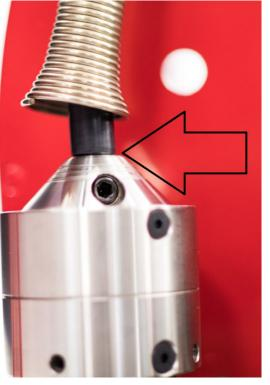
Step 6. Connect the Shaft to the Safety Clutch and tighten the Hex Socket Set Screws (2pcs) with a Hex Key 4mm. The Outer casing should almost touch the Safety Clutch, bare cable is always weak and therefore can twist.
